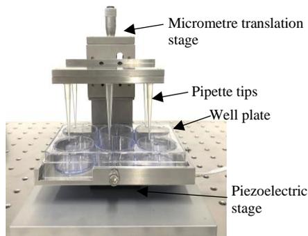
Figure 1 Developed scratch assay apparatus.
